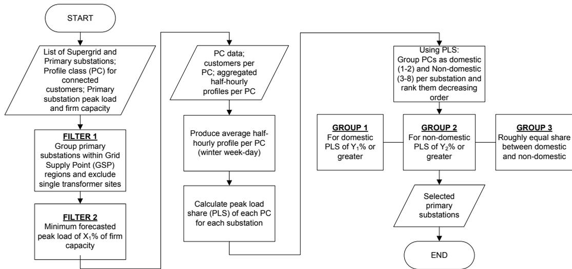
Figure 1: Flowchart showing methodology for selecting Primary substations for CLASS trials
