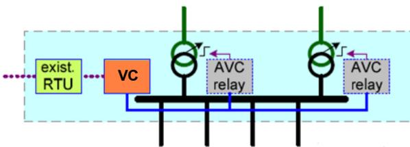
Figure 4 - Siemens plc Voltage Controller (VC) alongside existing infrastructure
