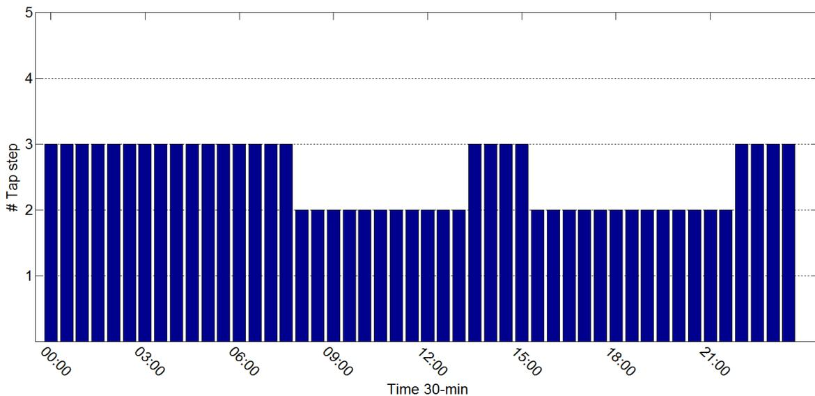
**Figure 11 Potential number of tap changes for voltage reduction purposes in Romiley primary (3<sup>rd</sup> September)**
