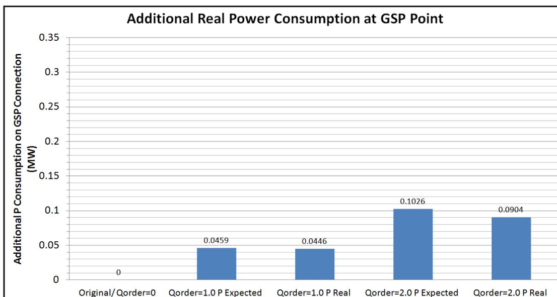
Figure 20: P changes at the power source point due to tap staggering
