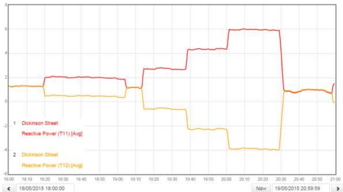
**Figure 4-15: Reactive power outputs measured at the secondary sides of the Dickinson St substation**
