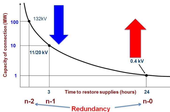
Figure 15.5: Paradigm shift in network design philosophy enabled by web-of-cells / microgrids structures
