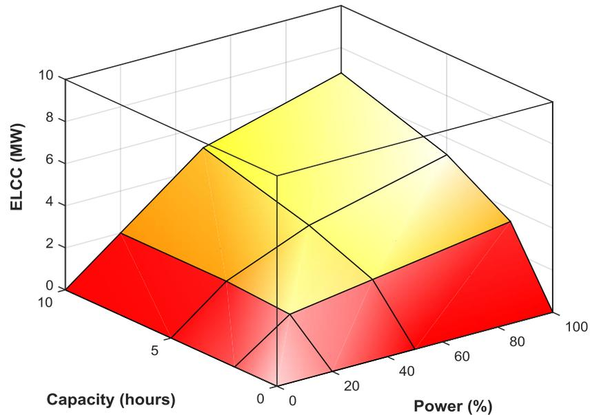
Figure 7.5: ELCC for different storage plants under reliability scenario MTBF = 1 year and MTTR = 3 hours. N-1 level of network redundancy.
