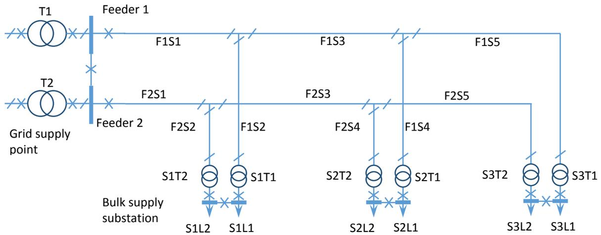
Figure 5.8: The illustrative topology of a 132 kV network with 3 bulk supply substations used in the study
