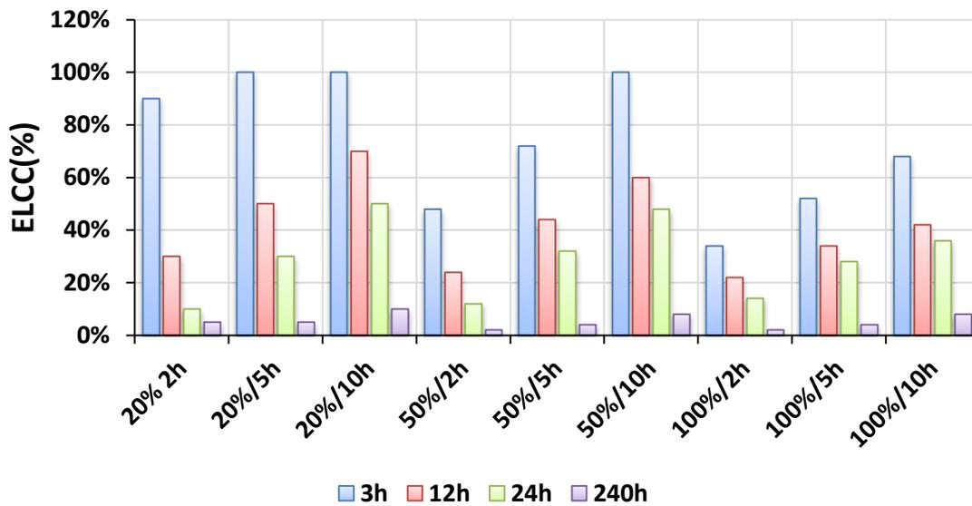
Figure 7.6: Normalized ELCC for storage plants of different sizes across four reliability levels under the N-1 network redundancy scenario.
