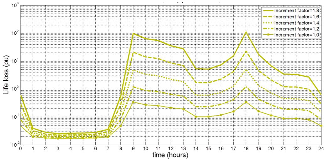
Figure 9.3: Impact of increasing utilisation of a cable on its lifetime
