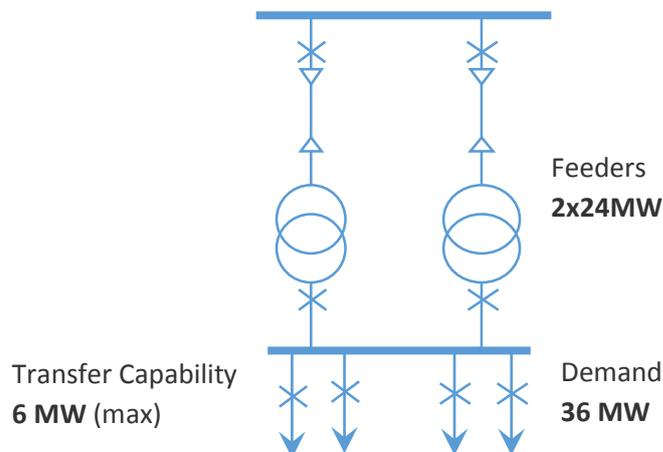
Figure 5.4. Dual-circuit transformer-feeder system
