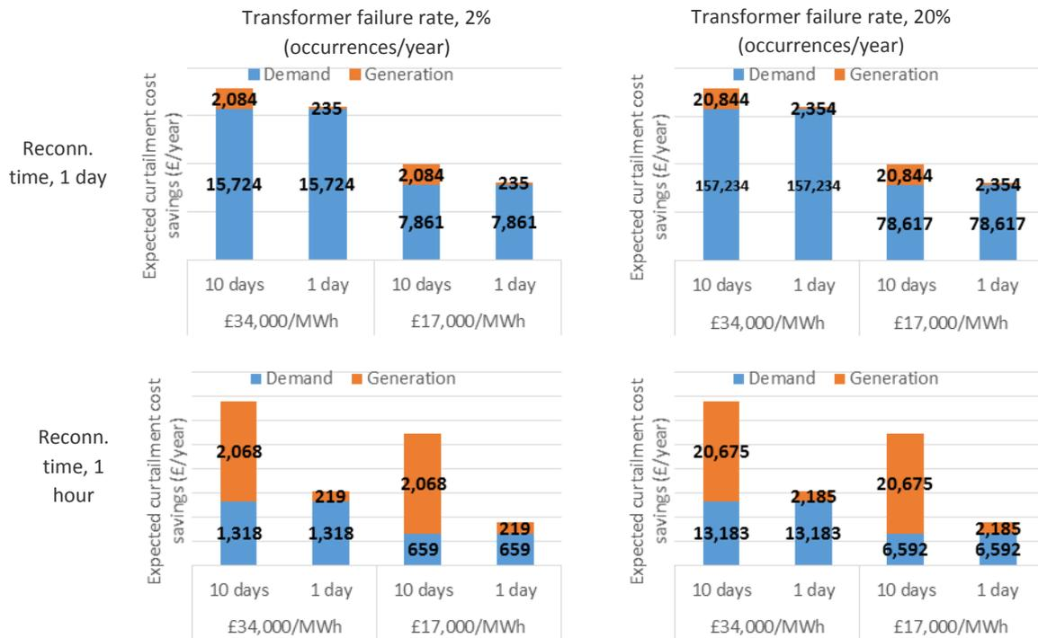
Figure 6.2: Savings in curtailments costs from installing a third transformer
