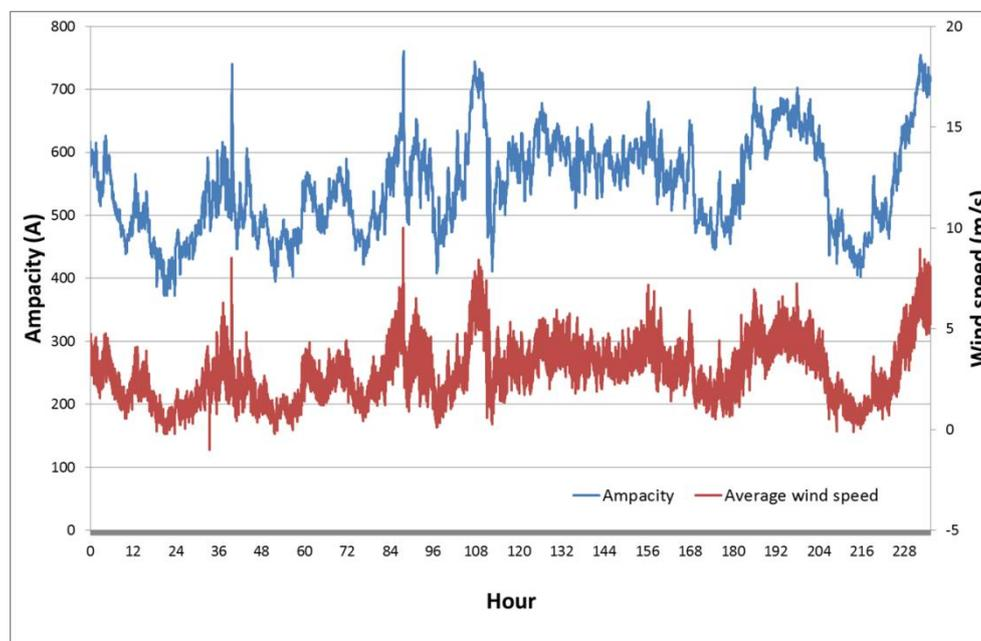
Figure 9.1: Real-time ampacity of OH lines and wind speed over a period of 10 winter days
