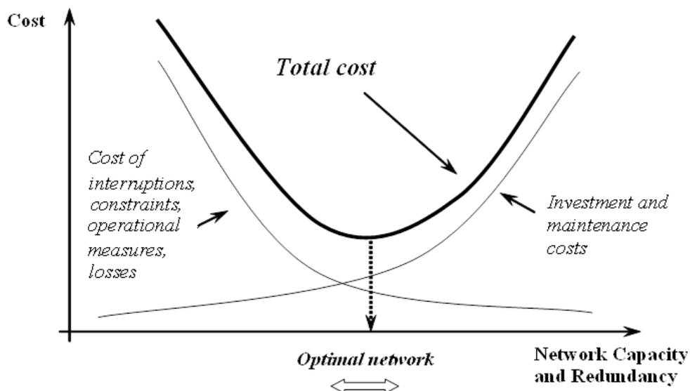
Figure 4.1: Probabilistic cost-benefit analysis framework for distribution network operation and planning
