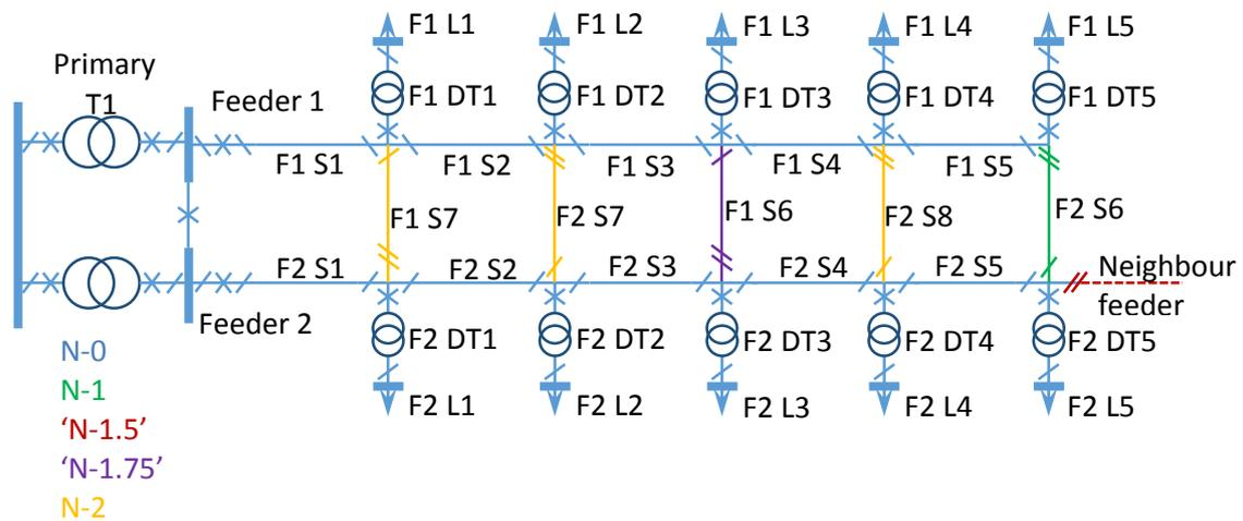
Figure 15.2: A generic HV network system with different configurations to provide certain levels of security of supply
