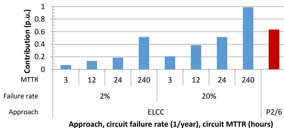
Figure 7.2: Illustration of security contribution of demand or generation led DSR
