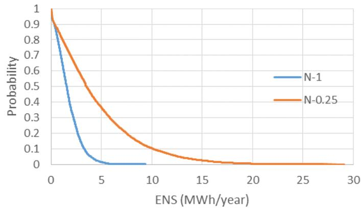
Figure 5.3. Cumulative probability of ENS for case C with switching time of 30 minutes
