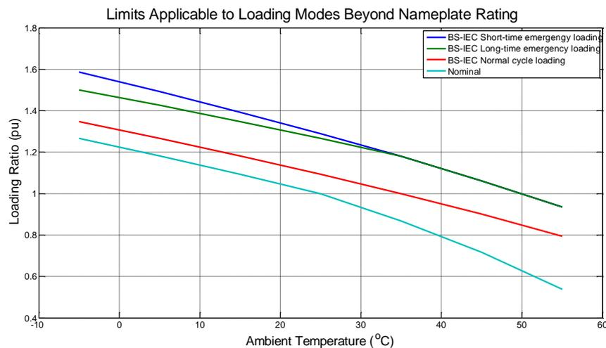
Figure 9.2: Maximum transformer’s loading capability for various loading modes
