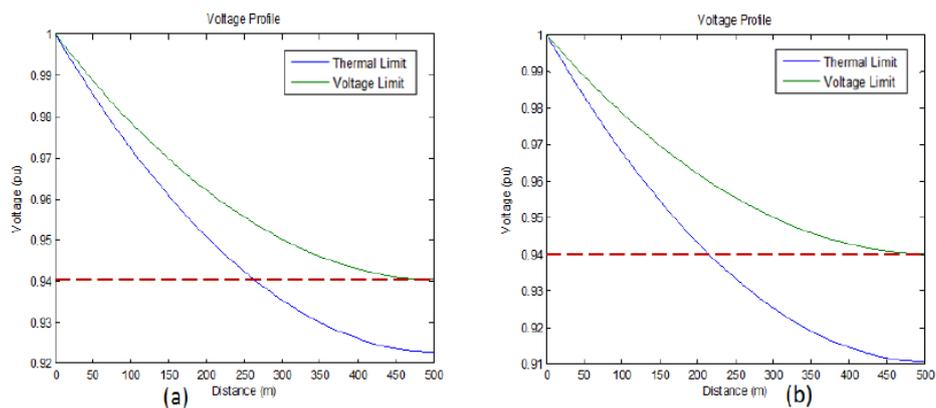
Figure 9.4: Voltage profiles for LV feeders with (a) 300 mm<sup>2</sup> and (b) 185 mm<sup>2</sup> cables under different loading conditions
