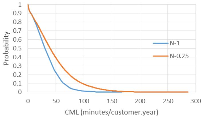
Figure 5.2. Cumulative probability of CML for case C and switching time of 30 minutes
