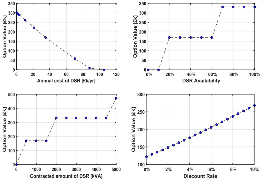
Figure 13.3: Impact of cost of DSR, availability of DSR, contracted amount and discount rate on the option value of DSR
