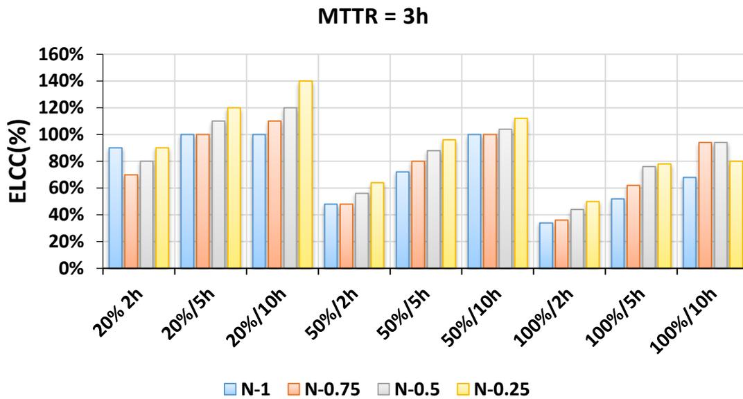
Figure 7.7: Normalized ELCC for storage plants of different sizes across four network redundancy levels when transformers' MTTR = 3 hours.
