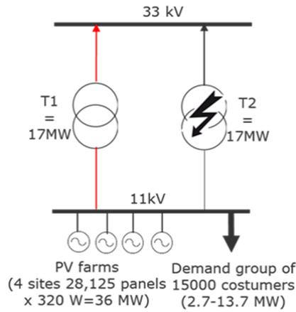
Figure 6.1: A failure in T2 in combination with reverse flows may overload T1
