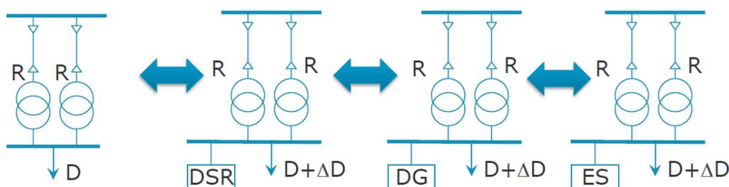
Figure 7.1: The basic concept for assessing the security contribution of DER
