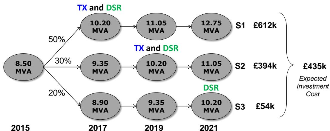
Figure 13.2: Optimal investment strategy when the planner can build both conventional and DSR assets.
