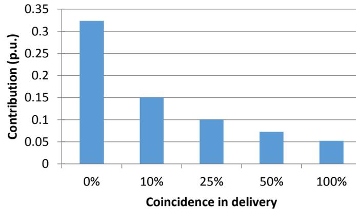
Figure 7.4. Illustration of impact of coincidence in delivery on DSR contribution
