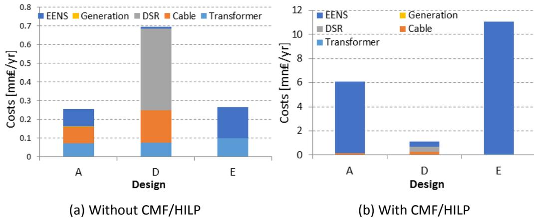
Figure 11.2: Cost components of each option in conditions without and with CMF/HILP
