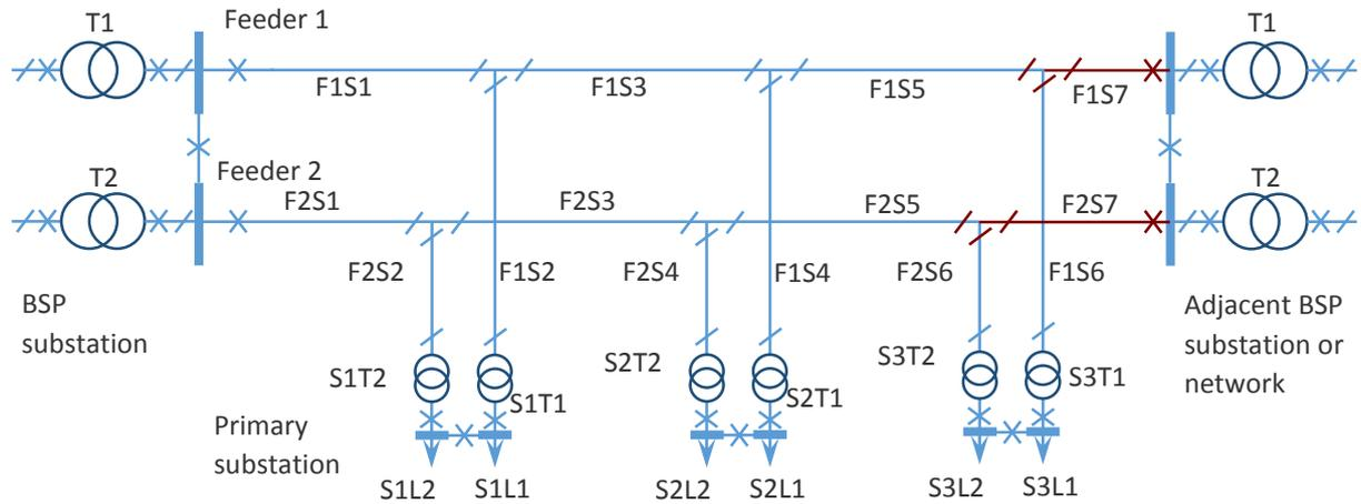
Figure 15.4: EHV Generic network configurations (Three Primary Substations Illustration)
