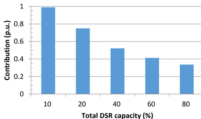
Figure 7.3. Illustration of impact of relative size of DSR on its contribution
