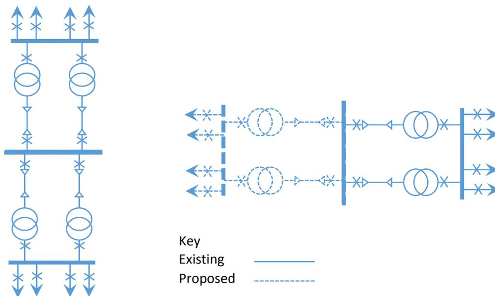
Figure 5.6. Schematic layout of 33/11 kV substations
