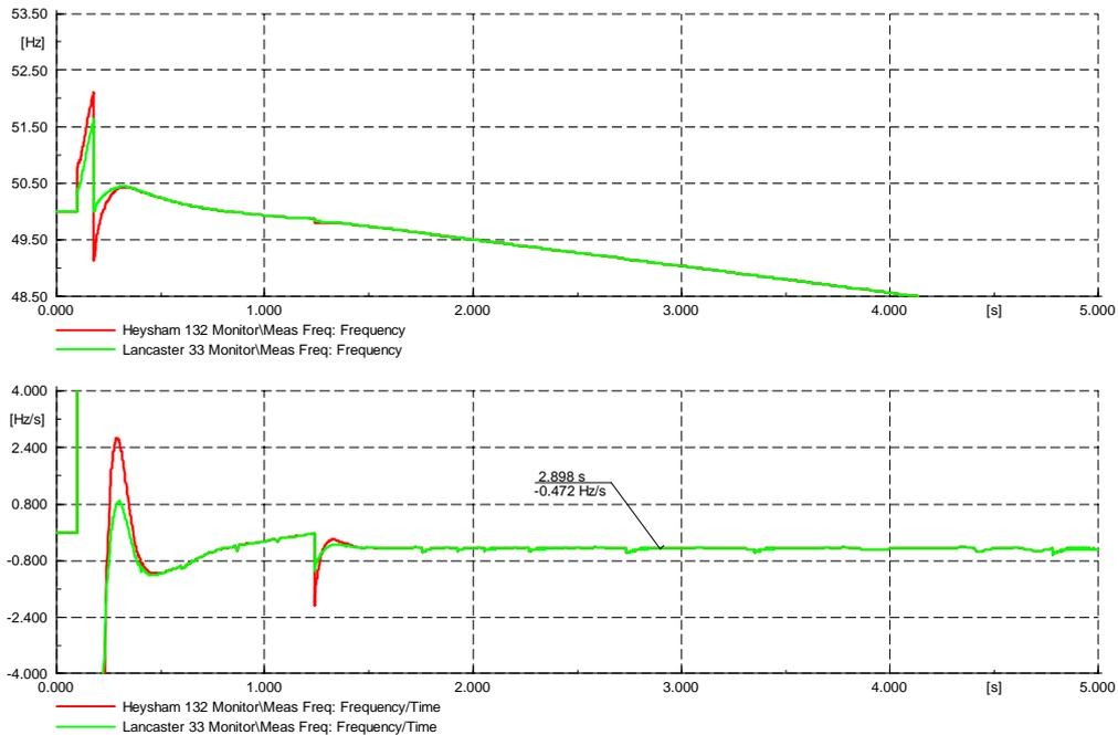
To resolve this, the voltage setpoint of the SGTs at Heysham GSP was reduced from 1.03 to 1.01 pu and wind machines set to voltage control mode in the initial condition. In this case the frequency after 5s is 49.89 Hz as shown in Figure 6 .
