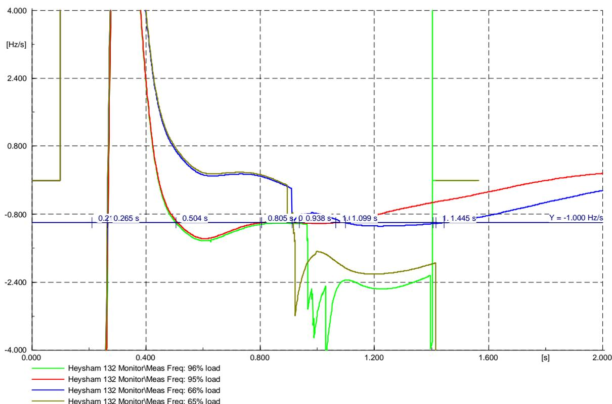
The events described for 110ms are common to all intertrip times tested up to 140ms. It was not possible to facilitate an intertrip delay of 150ms in this scenario.
