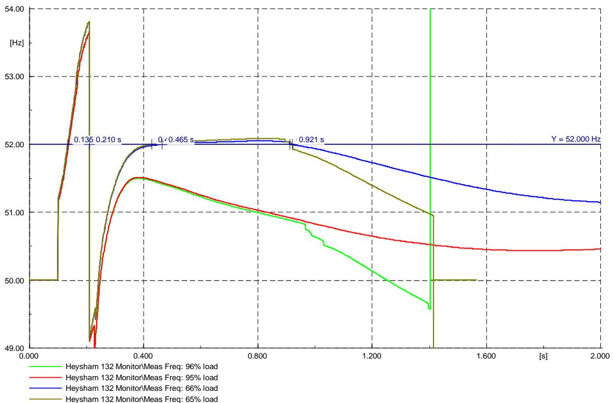
Figure 22 - Rate of Change of Frequency [Hz/s] at Heysham 132kV bus when facilitating a 110ms intertrip delay time
