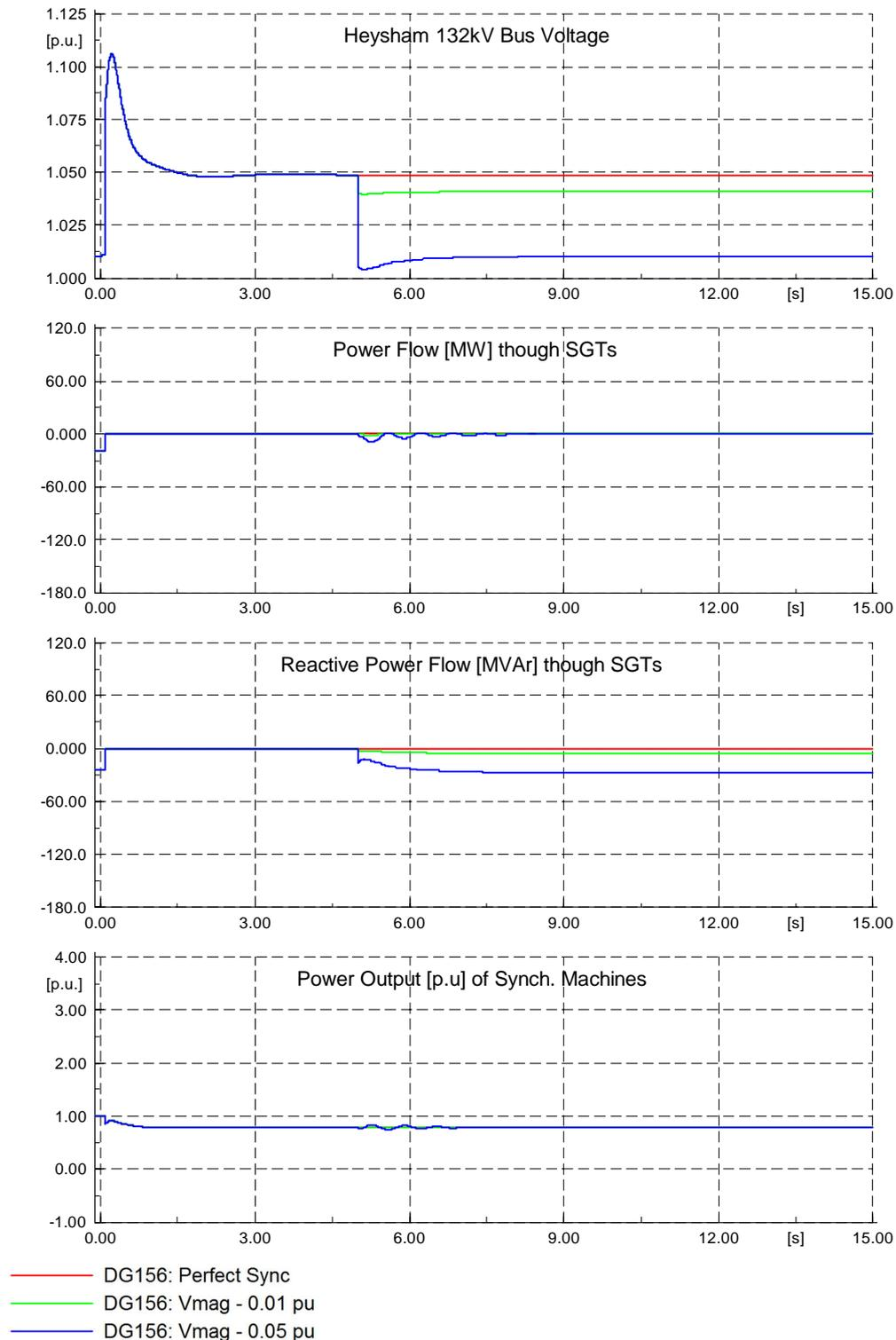
Phase Angle difference is the time in electrical degrees between the zero crossings on the voltage of the two systems. A phase angle difference will cause a sudden MW flow to appear across the closing circuit breaker. The Figure 27 below shows the response when the phase angle over the closing breaker is 10 degrees different. In this case, a transient power flow, peaking at 60 MW can be seen, before returning to zero in the steady state.
