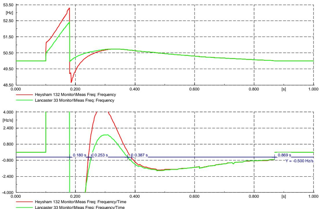
Further reducing demand to 80% or curtailing large wind machines to 60% of their output is sufficient to shorten the duration of frequency decline and prevent the medium machines from tripping on RoCoF within the first second. However, a subsequent transient overvoltage was found to cause one medium sized (8MW) plant to trip at  $t=1.25s$ ; which leads to frequency decline at around  $-0.47 \text{ Hz/s}$  and tripping of remaining machines on under frequency. This can be seen in Figure 5 below.
