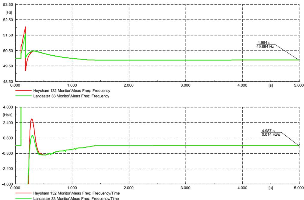
After applying the homogenous RoCoF settings stated in G99, the small plant (<5MW) will remain connected when the islanding breaker opens; and more medium size synchronous generation will remain connected within the first second. As such, the limitations on load is removed i.e. the network can maintain 100% peak demand, and there is no requirement to curtail any generation. In this case there is a slight steady state over frequency at 50.5 Hz, and 132kV system voltage is less than 1.045 p.u.
